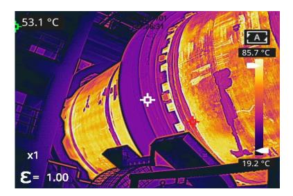
**Rotary Kiln Defect Monitoring**
