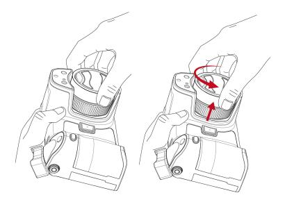
2. Carefully pull out the lens from the lens bayonet mount.
