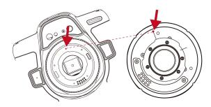
5. Align the lens correctly to the bayonet mount. Carefully push the lens into position.
